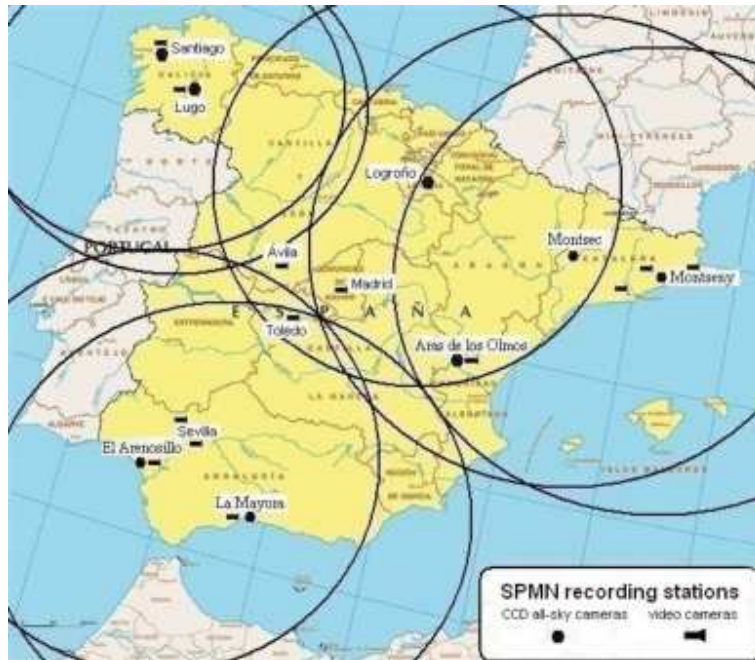
Figure 1.— The SPMN stations currently operating with the different imaging systems that are being used also shown. The circles represent the 400-km wide fireball detection areas optimally covered from each station, although the detection limit for bright bolides is about 550 km.
